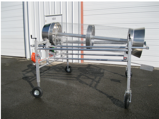
Wide Frame 2420 with Straight Mount Tires on Input End (Standard) & Swivel Tires on the Output End and Diverter
